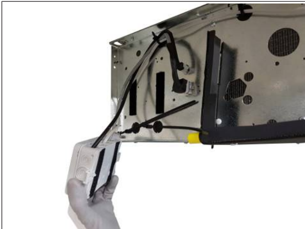
Fig. 43: Remove junction box from the Velcro strip
