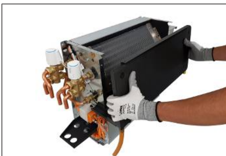
Fig. 72: Removing the main condensation tray
