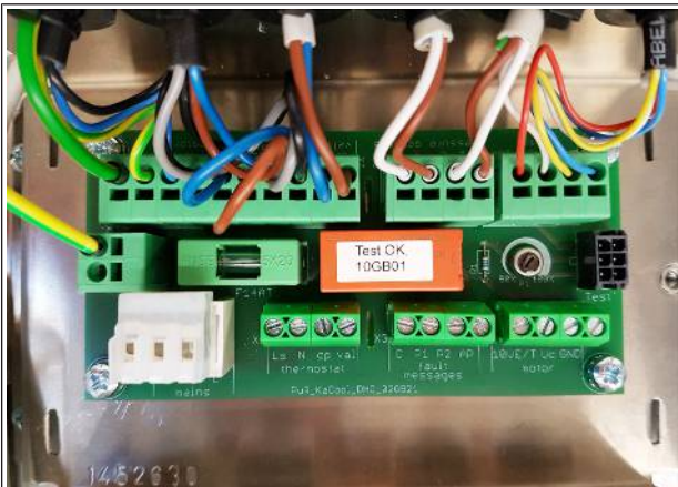
Fig. 12: PCB in the electrical junction box
